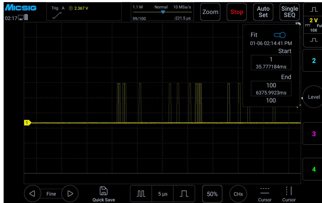
Figure 12-13 Segmented storage fitting view
