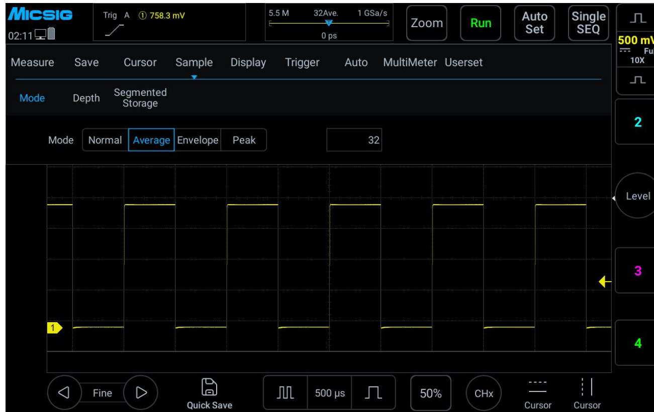
Figure 12-5 The waveform after selecting the average sampling mode, with the average number being 16.
